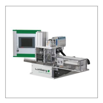
Semiautomatic harnessing machine for termination of RAST 2.5 Power connectors in insulation displacement technology (IDT)
