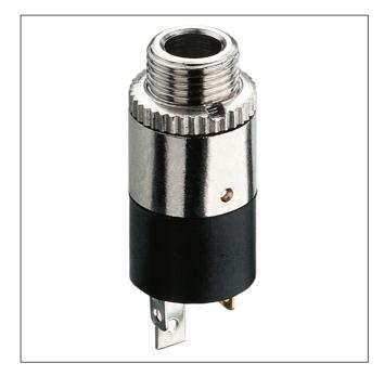
Jack chassis socket acc. to JIS C 6560 JC35J3A, 3.5 mm, 3 poles/stereo, with solder eyes, for back side mounting
