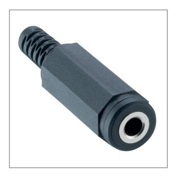
Jack socket acc. to JIS C 6560 JC35J2A, 3.5 mm, 2 poles/mono, straight version, with bend protection and solder terminals
