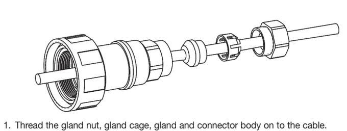
1. Thread the gland nut, gland cage, gland and connector body on to the cable.
