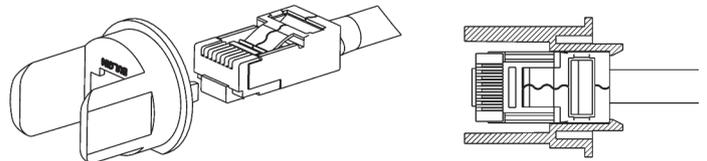
6. Push the RJ45 into the carrier moulding until it latches.
