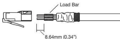
4. Push load bar and cable fully home into RJ45, ensuring the braid and foil are in contact with the metal shell. Crimp RJ45 with appropriate crimp tool and die set. Trim back braid and foil flush with rear of RJ45 body.
