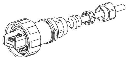
8. Slide gland, gland cage and gland nut up to body moulding then tighten to torque of 1.5-2.0lb/ins, 13-18Nm.
