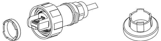
7. Pull up the connector body and locate the carrier. The carrier sits into a 'D' shape aperture in the connector body, ensure it is seated correctly. Locate locking ring and tighten ring to retain insert, using the assembly tool provided.
