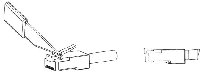
5. Crop the latching clip on the RJ45 ensuring this is completely removed.
