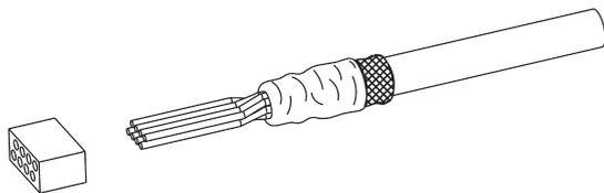
3. Un-twist the conductors and feed through the appropriate hole in the load bar, according to the wiring standard required. Push the loading bar fully home on to cable. Trim conductors to extend 8.64mm (0.34") out of the front of the load bar.
