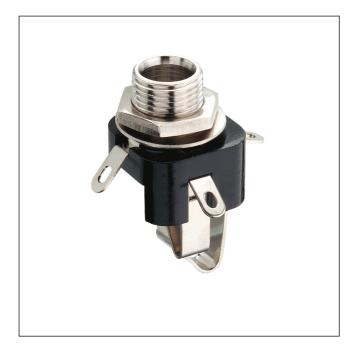
Jack chassis socket acc. to JIS C 6560 JC63J3A, 6.35 mm, 3 poles/stereo, with solder eyes, for back side mounting
