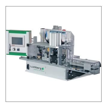
Semiautomatic harnessing machine for termination of RAST 2.5 connectors in insulation displacement technology (IDT), larger base machine, with integrated stations for cable color detection, keying cutting and keying testing, individual upgrading possible
