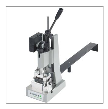
Knuckle-joint press for termination of RAST 2.5 Power connectors in insulation displacement technology (IDT)
