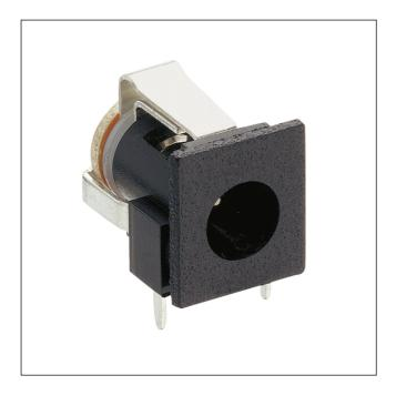
Power supply chassis socket acc. to DIN 45323, angular version, with flange and break contact, for printed circuit boards
