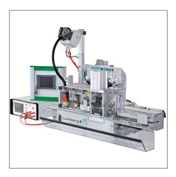
Semiautomatic harnessing machine for termination of RAST 2.5 connectors in insulation displacement technology (IDT), larger base machine, with integrated stations for cable color detection, keying cutting, keying testing and high-voltage test
