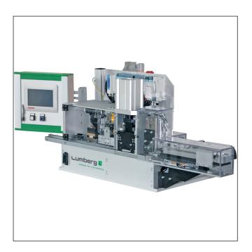
Semiautomatic harnessing machine for termination of RAST 2.5 Power connectors in insulation displacement technology (IDT), larger base machine, with integrated stations for cable color detection, keying cutting and keying testing, individual upgrading possible
