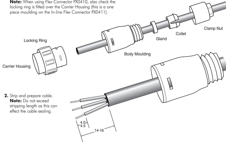
2. Strip and prepare cable. **Note:** Do not exceed stripping length as this can effect the cable sealing.
