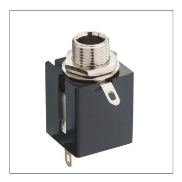
Jack chassis socket acc. to JIS C 6560 JC63J3Z, 6.35 mm, 3 poles/stereo, with break contact and solder eyes, for back side mounting
