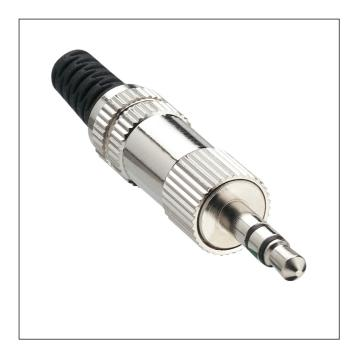
Jack plug acc. to JIS C 6560 JC35P3, 3.5 mm, 3 poles/ stereo, straight version, with metal housing, bend protection and solder terminals
