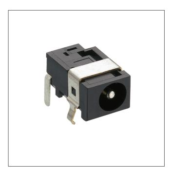
Power supply chassis socket acc. to JEITA RC-5320A JSAJ31, angular version, with break contact, for printed circuit boards
